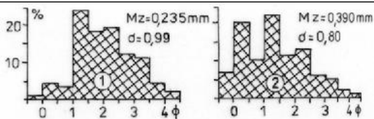
Fig. 4. Grain size distribution of sandy deposits of Barguzin Basin: 1 – kuytun deposits, 2 – presents aeolian sands
